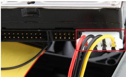
Locate the IDE data cable. Connect it to the IDE data port on your drive.
